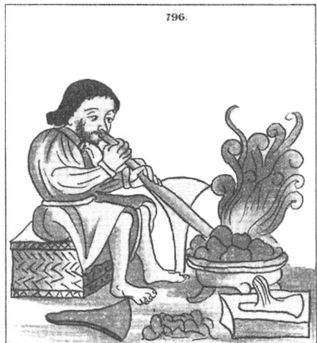
Figure 8. An Aztec metalworker casting axes using a crucible with a spout and a clay mold (redrawn from Sahagún 1950–1975:11:Plate 796).
